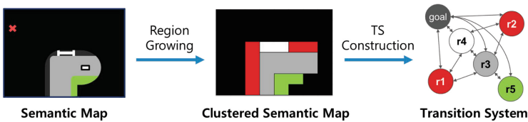
Fig. 3. Transition system formulation process. A region growing algorithms clusters regions with identical labels. A transition system then represents the connections.
